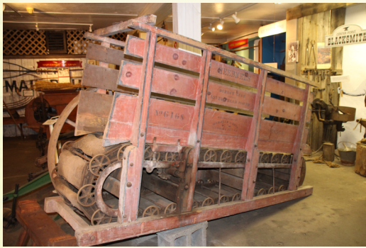
Heebner Direct-Geared, One Horsepower, Tread Mill at its current home in the Bill Bourne Farm Museum.
